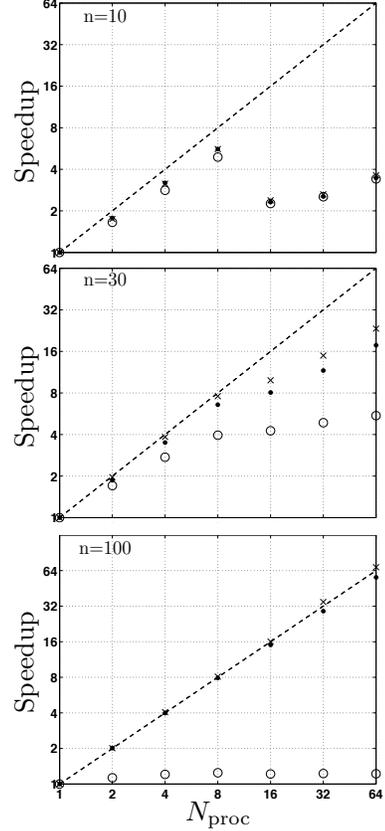
**Figure 4: Parallel speedup  $s$  of the parallel CMA-ES ( $\bullet$ ), and PS-CMA-ES with constant ( $\circ$ ) and decreasing ( $\times$ ) number of MPI communications on the random landscape test problem in  $n = 10, 30, 100$  dimensions. The number of processor cores  $N_{\text{proc}}$  is varied from 1 to 64. Each point is averaged from  $R = 5$  runs. Error bars are comparable to symbol size and therefore not shown.**
