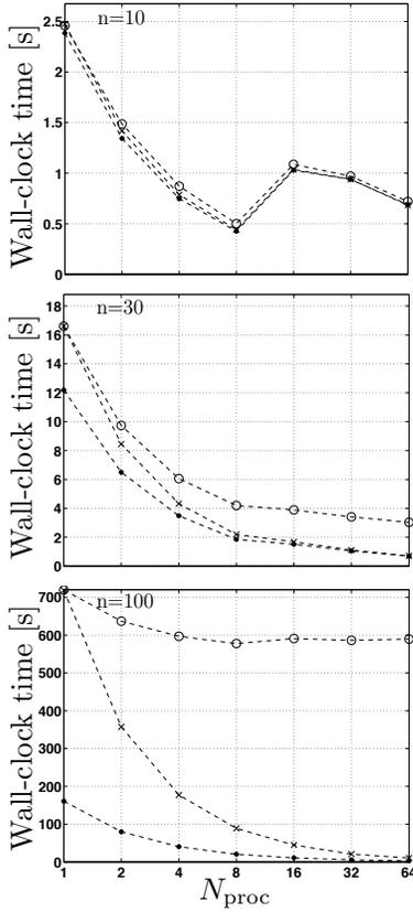
**Figure 3: Overall run time  $t(N_{\text{proc}})$  in seconds for the parallel CMA-ES ( $\bullet$ ), and PS-CMA-ES with constant ( $\circ$ ) and decreasing ( $\times$ ) number of MPI communications on the random landscape test problem in  $n = 10, 30, 100$  dimensions. The number of processor cores  $N_{\text{proc}}$  is varied from 1 to 64. Each point is averaged from  $R = 5$  runs. Error bars are comparable to symbol size and therefore not shown.**
