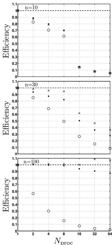
**Figure 5: Parallel efficiency  $e$  of the parallel CMA-ES (●), and PS-CMA-ES with constant (○) and decreasing (×) number of MPI communications on the random landscape test problem in  $n = 10, 30, 100$  dimensions. The number of processor cores  $N_{\text{proc}}$  is varied from 1 to 64. Each point is averaged from  $R = 5$  runs. Error bars are comparable to symbol size and therefore not shown.**
